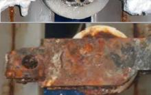
**BODY**: Plating is corroded, serious white rust. **BAR**: Plating is corroded, rust is present.
